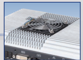
With external fan installed
